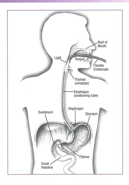
**An endoscope** is a flexible tube about half an inch in diameter and between 3 and 5 feet long. Fiber optics carry light down to illuminate the area being examined, and carry a clear image back to the eye piece. In some cases a camera sends images back to a TV monitor.
